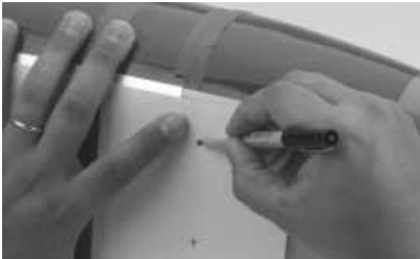
**Step 6.** Using a 1/16" drill bit, carefully drill the four cowl mounting screw locations. Drill through the cowl and into the plywood fuselage doubler (approximately 1/2").
