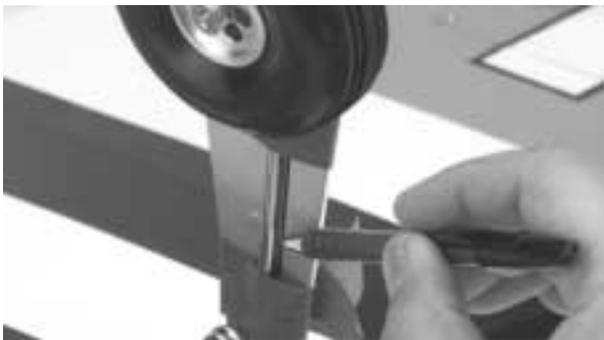
**Step 7.** Turn the fairing over and draw a line from the top to the bottom. Measure in 2" from both the top and the bottom and mark the location for the mounting straps.
