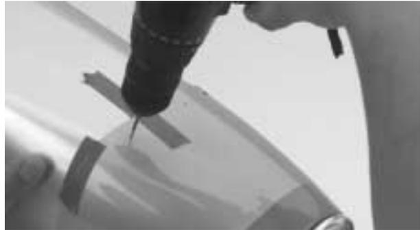
**Step 7.** Mount the cowl using the #2 wood screws provided.
