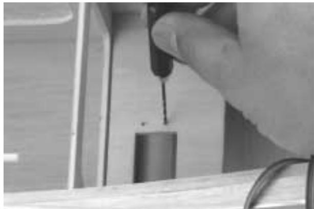
**Step 8.** Mount the throttle servo using the screws provided with your radio system. The throttle linkage will be installed later in this manual.
