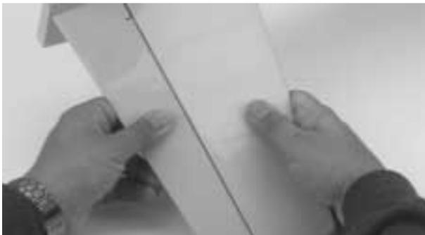
**Step 7.** Once the epoxy has cured, deflect the elevators down and use a high-quality thin CA to completely saturate each hinge.
