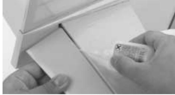
**Step 8.** Turn the fuselage over and repeat the hinge gluing process by deflecting the elevators in the opposite direction and again completely saturating each hinge with thin CA. Wipe away any excess CA using CA Remover/Debonder and a paper towel. Allow the CA to completely dry.
