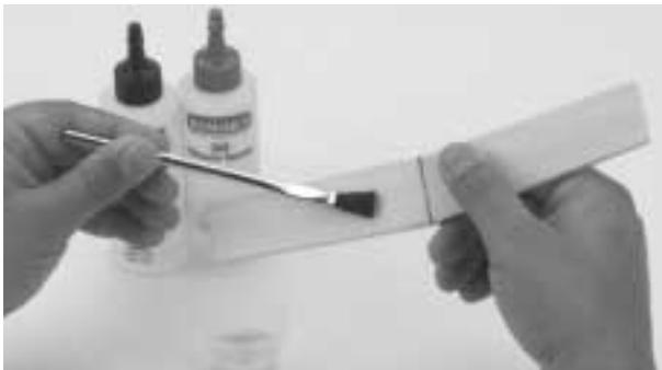
**Step 6.** Apply a generous amount of epoxy to the other wing panel joiner cavity.
