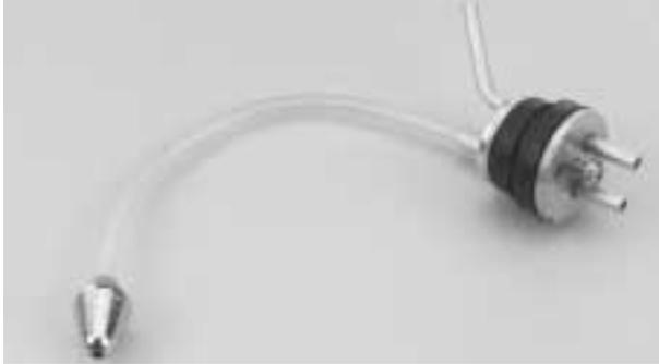
**Step 7.** Carefully insert the assembly into the fuel tank. Note the position of the vent tube; it must be at the top portion of the fuel tank to function properly. Also, it may be necessary to shorten the length of the fuel pickup tubing to make sure the clunk does not rub against the back of the fuel tank. You should be able to turn the tank upside down, which allows the clunk to freely drop to the top of the tank.
