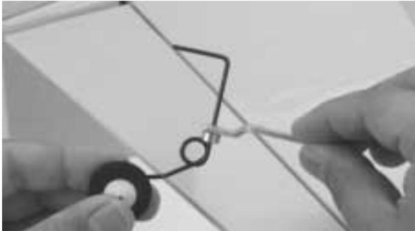
**Step 2.** Temporarily install the rudder using the hinges provided; do not glue the hinges at this time. Hold the tail wheel assembly up to the fuselage as shown and mark the location where the wire will insert into the rudder. Remove the rudder.
