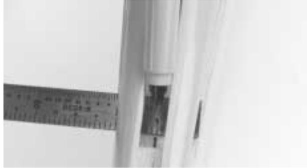
**Note:** The horizontal stabilizer is positioned all the way forward in the saddle area to allow room for the elevator joiner wire. The wire will be inserted through the saddle area before the horizontal stabilizer is glued in place.
