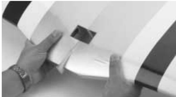
**Step 3.** Check for correct dihedral angle. Place the wing on a large flat surface with one wing panel resting flat on the surface the opposite wing panel should be  $5\frac{1}{4}$ " from the flat surface (see illustration below). If necessary, sand the wing joiner until the proper dihedral is achieved. There should be no gap at the wing center joint. Once you are satisfied with the fit, separate the wing panels and remove the wing joiner.
