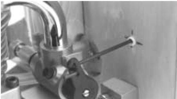
**Step 8.** Mount the EZ connector to the servo arm supplied with your radio system as shown. Connect the throttle servo to your radio system and center the throttle stick. Slide the EZ connector through the wire and mount the arm to the servo.
