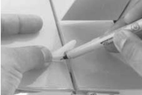
**Step 7.** Drill these holes with a 1/16" drill bit and install the rudder control horn, using the screws and backplate provided.
