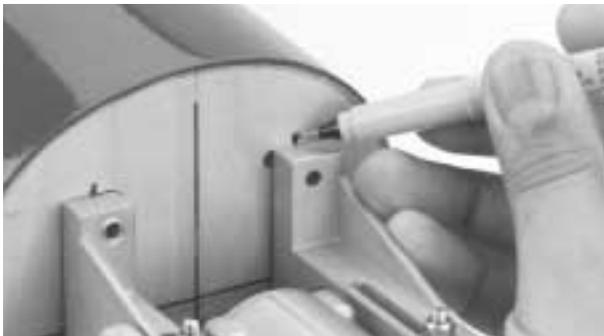
**Step 3.** Install the 8-32 blind nuts from inside the fuselage and mount the rails to firewall. Seat the blind nuts by tightening the bolts. Remove the bolts and carefully glue the blind nuts in place with Thin CA, be sure not to get any CA on the threads of the blind nuts.
