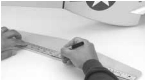
**Step 3.** Mark the center of the stabilizer saddle at the trailing edge of the saddle. You can hold the ruler at the back portion of the stab opening and use a pen or pencil to mark the center location through the opening of the vertical fin as shown.
