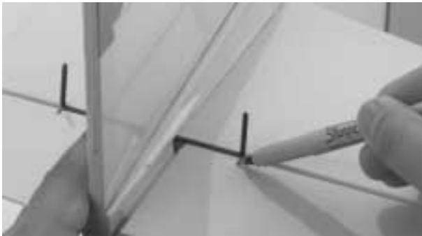
**Step 2.** Remove the elevators. Using a 3/32" drill bit, carefully drill the holes into the elevators using the marks you made in the previous step as a guide. Drill directly down the center of the elevator and only as far as needed.
