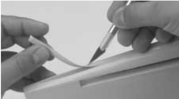
**Step 2.** Locate the horizontal stabilizer and elevator assembly and remove the elevators and hinges. Use a felt-tipped pen or pencil and ruler to mark the center of the stabilizer at the trailing edge as shown.
