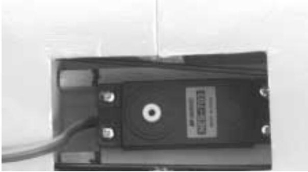
**Step 5.** Remove the retract servo from the mounting plate. Use thick CA and carefully glue the retract servo mounting plate to the servo rails. Align the plate with the marks you made on the rails. Allow the CA to fully dry before mounting to the wing assembly.
