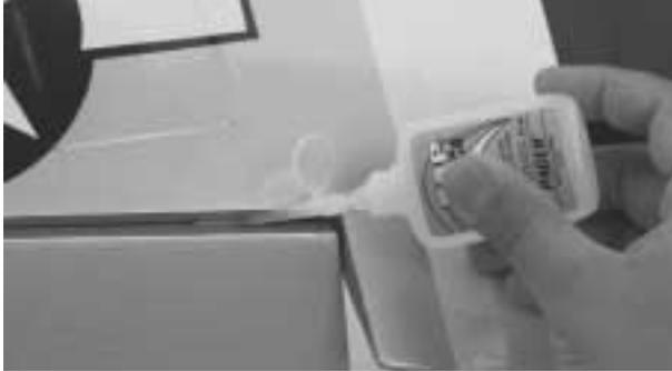
**Step 6.** Using CA remover/debonder and a paper towel, remove any excess CA glue that has accumulated on the wing or aileron surface.
