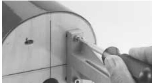
**Step 4.** Install the engine mount rails using threadlock and the 9/64" hex wrench. Loosely mount the engine to the rails and measure 5 $\frac{1}{4}$ " from the firewall to the prop drive washer of the engine. Tighten the mounting hardware and mark the location of the engine on to the mount. Use these marks to properly position the engine if it needs to be removed in the future.
