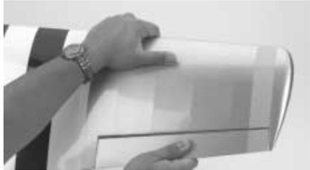
**Step 9.** Work the aileron up and down several times to “work in” the hinges and check for proper movement.
