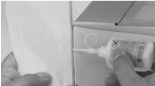
**Step 10.** Once the CA has completely dried, check the rudder for security by trying to pull the rudder from the fuselage. Use only enough pressure to test for security and be careful not to damage the wood structure of the rudder or fin.
