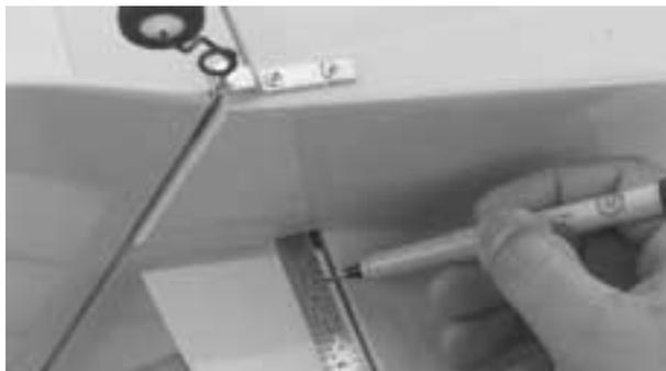
**Step 2.** Place the center of the control horn on the elevator at the mark made in the previous step. Mark the hole positions of the control horn with a felt-tipped pen or pencil.
