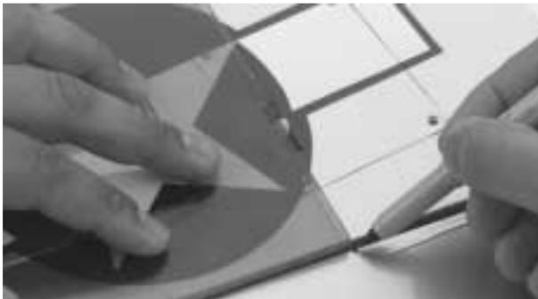
**Step 3.** Place the aileron control horn on the mark made in the previous step, aligning the center of the control horn on the mark. Also align the clevis holes in the horn with the aileron hinge line as show below and mark the location of the three mounting screws.
