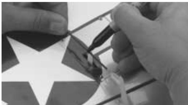
**Step 7.** Remove the clevis and wire from the control horn and make a 90-degree bend at the mark made in the previous step. Cut off the excess wire leaving 5/16" remaining after the 90-degree bend.
