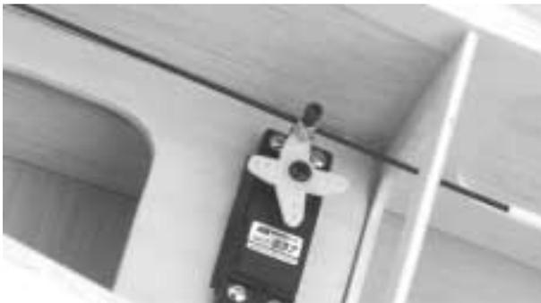
**Step 9.** With the throttle stick centered move the throttle arm on your engine to the center of its throw (1/2 throttle) and tighten the setscrew on the EZ connector. Trim off the excess wire.
