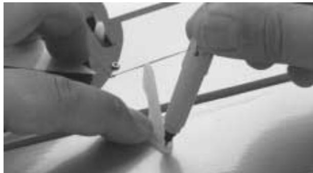
**Step 4.** With the mounting hole locations marked, drill the holes for the mounting screws using a 1/16" drill bit. Be sure to drill straight through the aileron at a 90-degree angle to the flat work surface not to the surface of the aileron.
