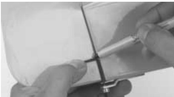
**Step 3.** Using a 3/32" drill bit, drill the rudder following the marks you made in the previous step. Make sure to drill straight into the rudder.
