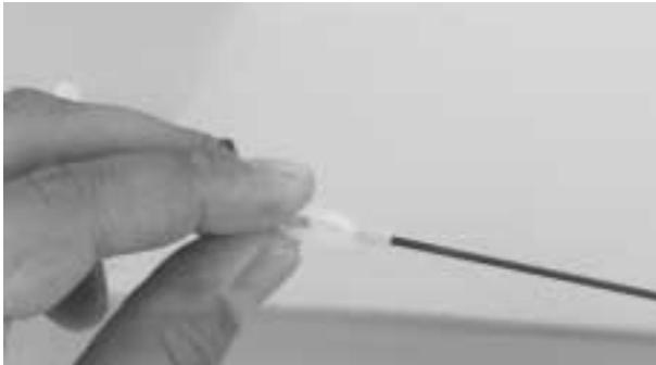
**Step 2.** Attach one clevis to the rudder control horn and, with the rudder centered and the servo electrically centered, mark the wire where it passes over the outermost hole on the servo arm.
