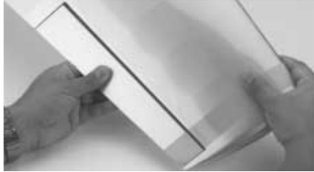
**Step 4.** Deflect the aileron and completely saturate the hinge with thin CA glue. Be sure not to deflect the aileron too far; the top of the aileron should just touch the top of the wing trailing edge. When the hinge is glued in place, there should be no more than a 1/32" gap maintained throughout the length of the aileron.
