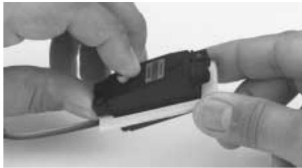
**Step 3.** Mark the location for the servo mounting screws using a felt-tipped pen or pencil. Remove the retract servo from the mounting plate and using a 1/16" drill bit, drill the holes for the servo mounting screws. Temporarily mount the retract servo to the mounting plate using the screws supplied with the servo.
