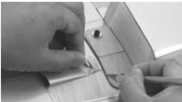
**Step 9.** Remove the wing and place a piece of wax paper or plastic wrap on the wing saddle where the radiator scoop contacts the fuselage. Remount the wing. Mix at least 1/2 ounce of 6-minute epoxy and coat both the radiator scoop and the wing. Align the radiator scoop with the fuselage and the bare wood exposed in Step 9. Secure the scoop in place using masking tape and wipe away any excess epoxy with rubbing alcohol and paper towels.
