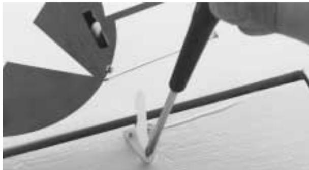
**Step 6.** Locate the aileron control wire (6" threaded on one end) and thread on a clevis a minimum of 12 turns. Attach the clevis to the middle hole in the control horn. To hold the aileron at the neutral position, place a piece of masking tape on the aileron to secure it to the wing trailing edge. With the aileron at neutral and aileron servo electronically centered mark the wire where it crosses the aileron servo arm.
