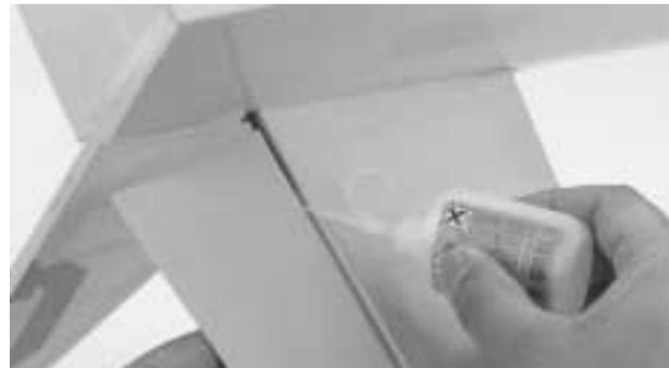
**Step 9.** Once the CA has dried, check the hinges for security by trying to pull the elevators from the stabilizer. Use only slight pressure and be sure not to crush the wood structure of the stabilizer or elevator.
