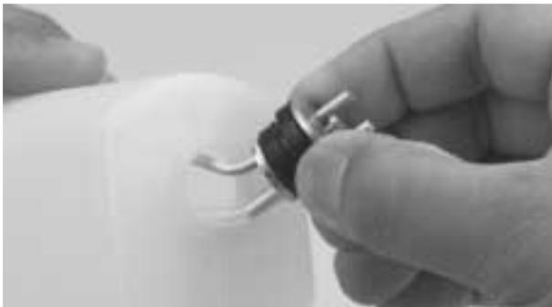
**Step 8.** Tighten the 3mm screw carefully—do not over tighten. This allows the rubber stopper to form a seal by being slightly compressed, thus sealing the fuel tank opening.
