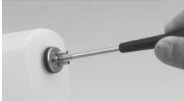
**Important:** Be sure to differentiate between the vent and the fuel pick-up tube. Once the tank is mounted inside the fuselage, it will be difficult to tell the tubes apart.
