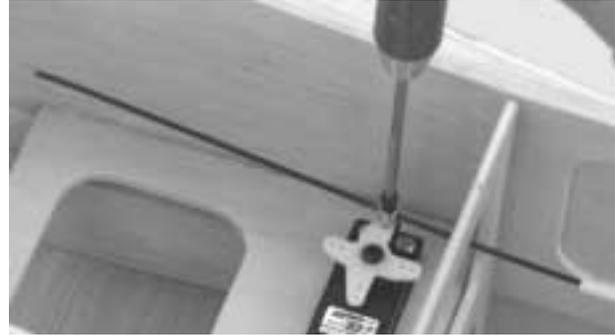
Check the throttle movement and adjust the end points if using a computer radio. If using a non-computer radio, adjust the end points by moving the connection of the wire either closer or further away from the center of the servo or throttle arm.
