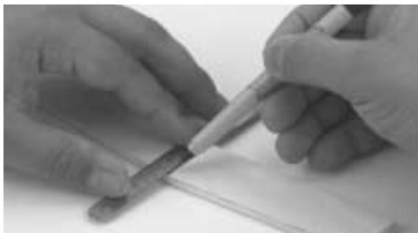
**Step 2.** Trial fit the wing joiner into one of the wing panels. It should insert smoothly up to the line marked in Step 1. Now slide the other wing panel onto the joiner until the two panels meet. If the fit is too tight, it may be necessary to lightly sand the wing joiner.
