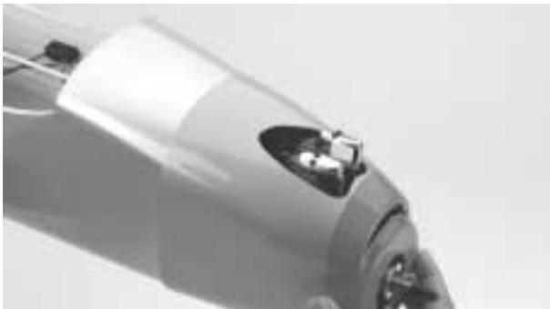
**Step 2.** Looking at the firewall, notice the plywood doubler on both sides of the fuselage. Measure 1/2" from the top and bottom of the doubler and mark with a felt-tipped pen, marking both sides of the fuselage. Measure 3/8" back from the firewall at the four marks you just made and make a mark. These are the cowl mounting screw locations.
