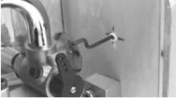
**Step 7.** Connect the Z-bend to your engines throttle arm. It may be necessary to remove the throttle arm to connect the throttle control wire.
