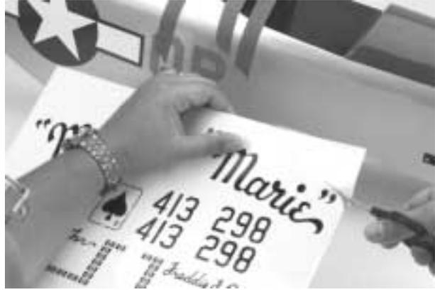
**Step 5.** Use the drawings to locate the position of the decals on the P-51. Use a water spray bottle with 2-3 drops of dish soap added to the water and spray both the fuselage and sticky side of the decal. This will allow you to reposition the decal if necessary. Once satisfied with the position use a paper towel to squeegee out the water. Allow the decal to dry over night.
