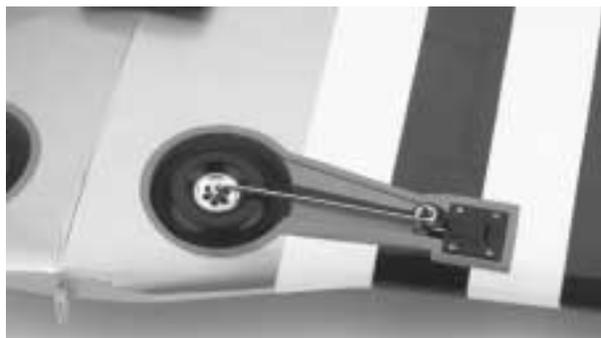
**Step 5.** Locate the landing gear fairing, two mounting straps, mounting screws, and nuts. Note that there is a left and right fairing. The outside of the fairing has white and black trim that matches the strips on the bottom of the wing.
