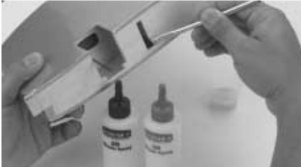
**Step 5.** Completely coat one half of the wing joiner with epoxy up to the centerline made in Step 1. Insert the epoxy-coated side of the joiner into the wing joiner cavity up to the mark on the joiner.
