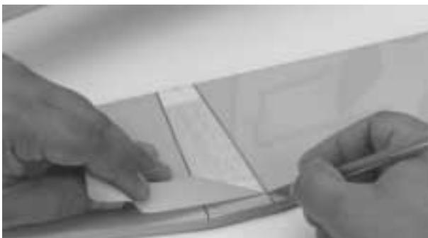
**Step 8.** Re-install the stabilizer into the fuselage. Use the lines drawn in Step 6 to reposition the stab correctly. Looking from behind the plane, check to make sure the horizontal stabilizer is parallel to the wing as shown in the illustration below. If any adjustments are required, lightly sand the stabilizer saddle to bring the horizontal stabilizer into alignment with the wing.
