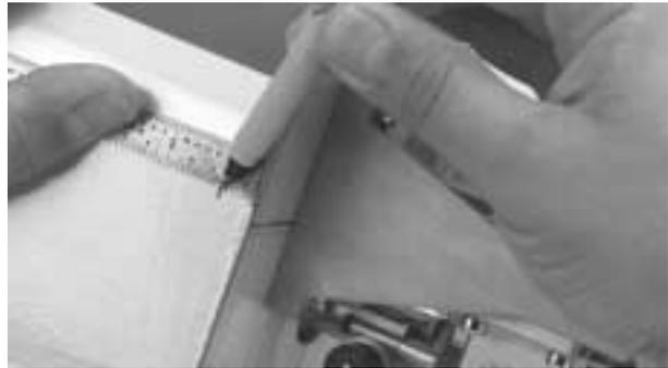
**Step 3.** To transfer these locations to the cowl, tape a piece of paper to the side of the fuselage as shown. Transfer the screw locations to the paper and fold back along the tape line.
