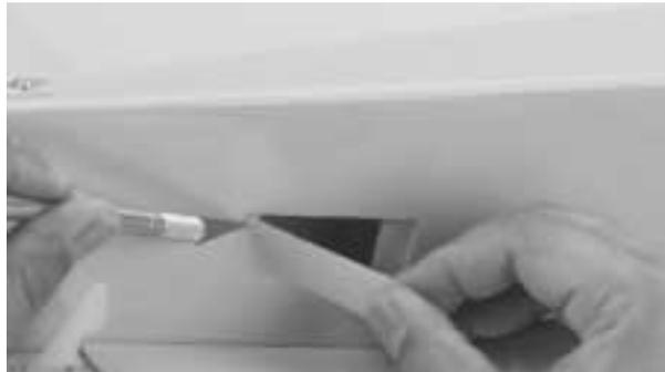
**Step 3.** Temporarily install the servos into the openings and mark the location of the servo mounting screws. Remove the servos and drill the holes for the servo mounting screws using a 1/16" drill bit.
