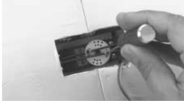
**Step 11.** Cycle the retract system several times and check to make sure there is no binding, also check that the landing gear locks in both the retracted and extended position.
