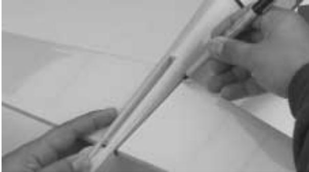
**Step 7.** Remove the stabilizer and use a sharp hobby knife to carefully remove the covering from the center of the stabilizer, cutting 1/16" inside the lines you marked in the previous step. Use only enough pressure to cut the covering and not the wood underneath, as doing so will severely weaken the structure of the horizontal stabilizer.
