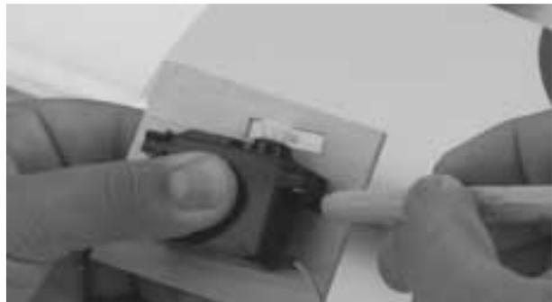
**Step 3.** Locate the servo mounting blocks. Using a few drops of thin CA, tack glue them in place on the marks made in the previous step. Check the fit of the servo between the mounting blocks. When satisfied with the fit, permanently glue the mounting blocks in place by first wicking thin CA between the mounting blocks and the hatch, and then using thick CA create a fillet around the base. Let the CA completely dry before proceeding to the next step.
