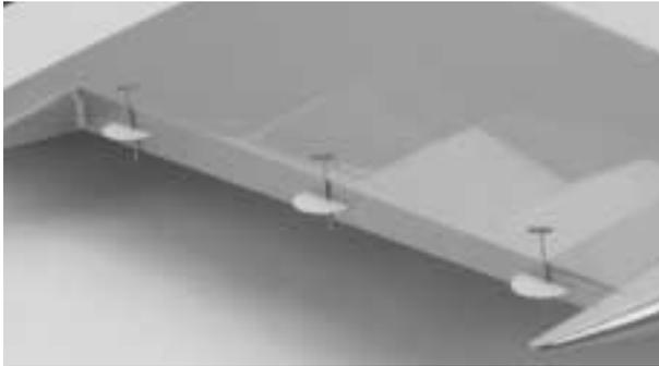
**Step 3.** Slide the aileron onto the wing until there is only a slight gap between the wing panel and aileron. The hinge is now centered in the wing panel and the aileron. You can now remove the T-pins and snug the aileron up against the wing panel.
