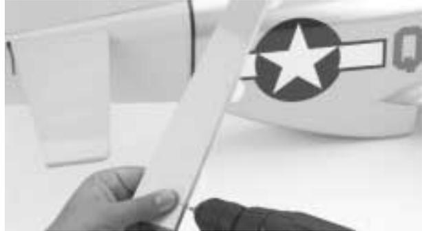
**Step 3.** Temporarily install the elevators back onto the horizontal stabilizer and check for fit. The elevator halves should be equal to each other and move freely up and down. If the elevators are not equal, you can remove them and carefully bend the joiner wire until they come into alignment. Once satisfied with the fit, remove the elevator halves.
