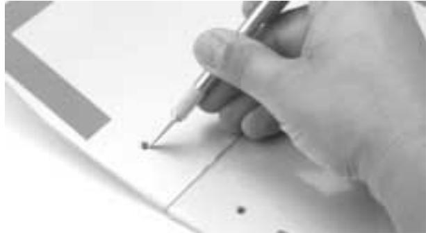
**Step 3.** Locate the plywood wing mounting plate. Align the plate with the trailing edge of the wing and the center joint as shown and mark the outline of the plate with a felt-tipped pen/pencil. Use a sharp hobby knife to trim away the covering 1/16" inside the lines you just drew.
