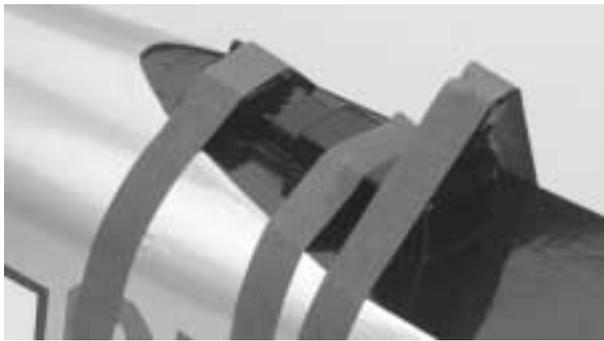
**Step 3.** Using the drawings, locate the position of the scale exhaust. It will be necessary to cut the exhaust pieces and glue one part to the fuselage and the other to the cowl. If necessary, cut an access hole for the cowl mounting screw before gluing on the exhaust.
