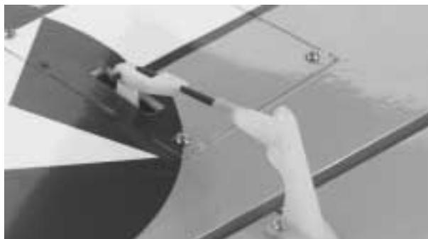
**Step 9.** Repeat Steps 1 – 8 for the opposite aileron control horn and linkage.
