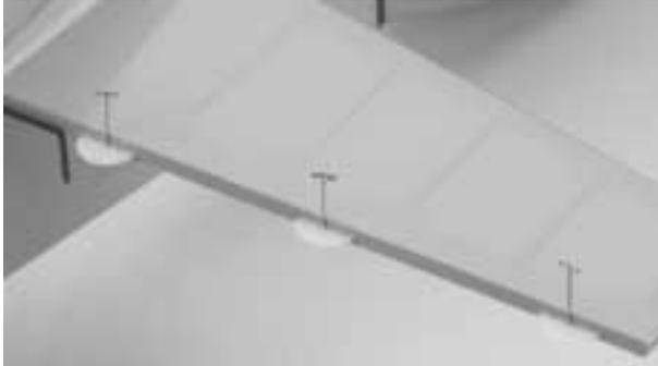
**Note:** In the following steps you will permanently install the elevators. Do not glue the hinges in place until the joiner wire epoxy has cured.
